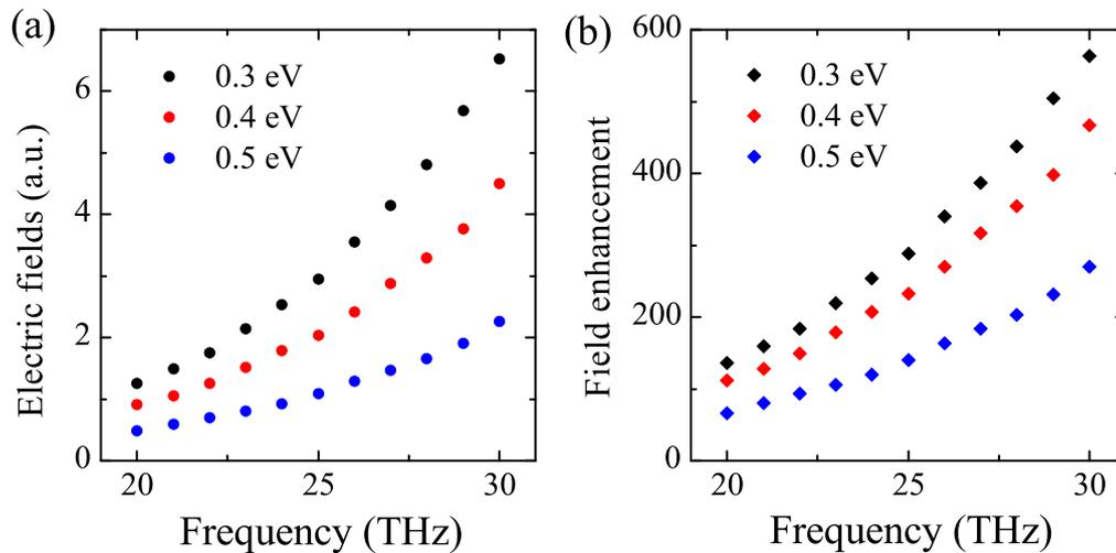
**Figure 4.** (a) Amplitudes of electric fields from 20 to 30 THz for different Fermi energies of graphene. (b) Field enhancement at the tip of the tapered graphene waveguide. Here, the field enhancement is defined as the electric fields at the tip of a tapered graphene waveguide divided by that at the edge of a 50 nm wide graphene ribbon waveguide under the same condition.
