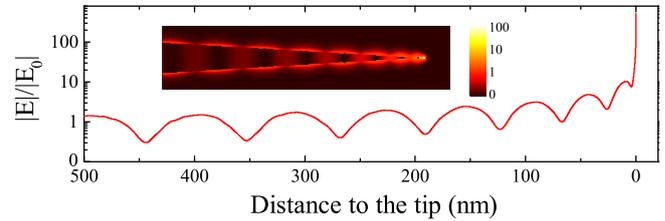
**Figure 3.** Amplitude of the local electric fields at one edge of a tapered graphene waveguide as a function of distance to the tip, normalized to that of a 50 nm wide graphene ribbon waveguide. The distributions of the amplitudes of the electric field at the tapered graphene waveguide is shown in the inset.
