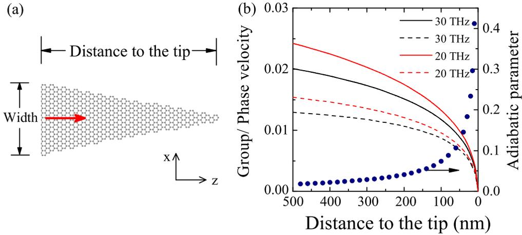
**Figure 2.** (a) Schematics of a tapered graphene waveguide. (b) Phase (solid lines) and group (dashed lines) velocities of two plasmon modes in a tapered graphene waveguide as a function of the distance to the tip. Circles represent the adiabatic parameter for a plasmon mode with a frequency of 30 THz.
